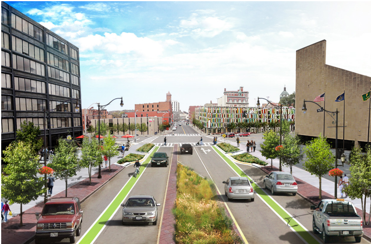
Rendering of proposed improvements at intersection of State & Hawley showing a narrowed gateway to slow speeds as drivers enter Downtown
