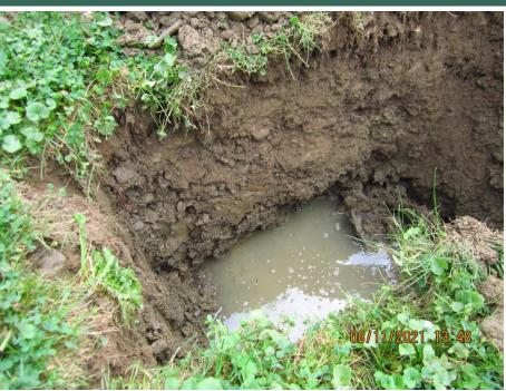
Various soil types in vertical soil profile (left). Groundwater encountered at shallow depth (right).
